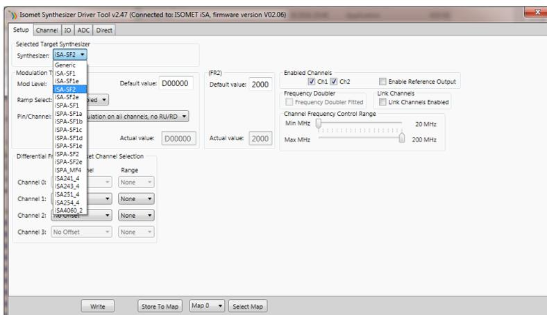
Certain models contain frequency doublers to extend the frequency range up to 400MHz. This option is factory fitted. The GUI allows for the multiplication provided the correct model is specified.
