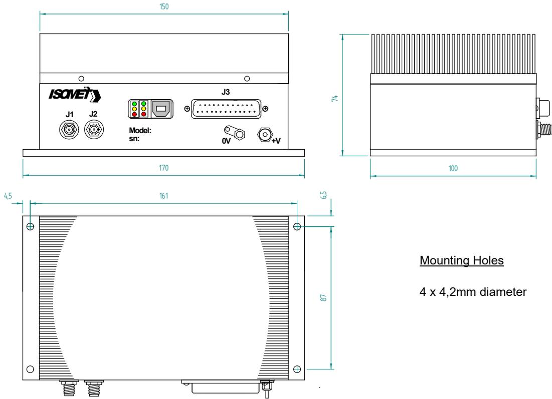
Figure 4a: Driver Installation, iSPA style shown with finned heat sink
